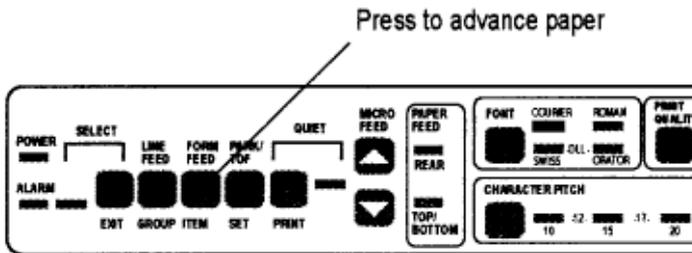
9. Set Top of Form (TOF) by holding PARK button while pressing appropriate MICRO FEED button. Paper will advance up or down in direction of arrow on button you're pressing. (For more details, see Setting Top of Form later in this chapter.)
