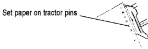
6. Push right lock lever back to lock tractor in position. Don't stretch paper tightly it can cause paper to tear.
