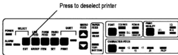
3. Press and hold PARK button while you adjust page up or down using MICRO FEED buttons. Red line on plastic ribbon shield marks base of printing line: use this as a guide.
