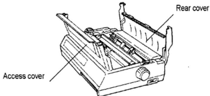
3. Use clean, dry cloth to dust area around carriage shaft and platen. Be sure to remove any loose particles of paper.
