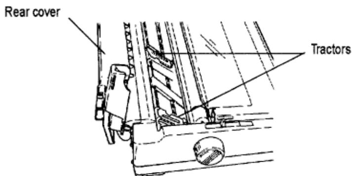
3. Open both tractor covers and pull forward on right-hand lock lever to unlock right tractor.
