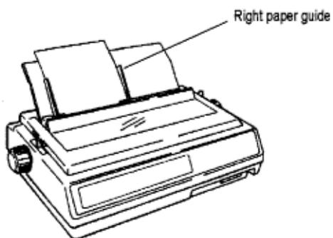
5. Press FORM FEED button to feed sheet into printer.
