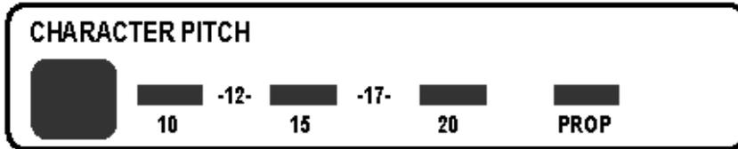
The character pitch determines the width of the individual characters and is measured in characters per inch (cpi).
