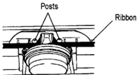
4. Unpack ribbon, remove its shipping restraint, and push idler roller latch in.
