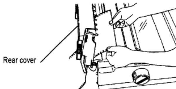
5. Slide right-hand tractor to adjust it to width of paper, then set paper on tractor pins at either end and
