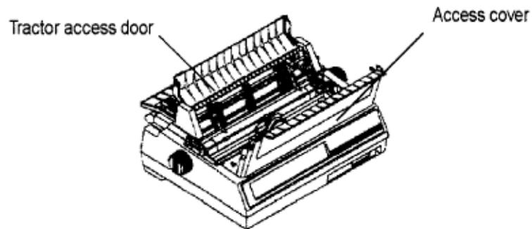
3. If you have bottom-feed push tractor unit installed, open the printer access cover and the tractor access door and remove any shreds of paper jammed in tractor mechanism.
