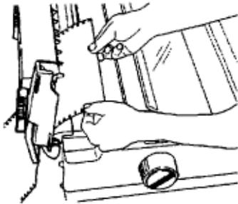
4. Fold some single-sheet, continuous-feed paper over three times to produce a page four sheets thick.
